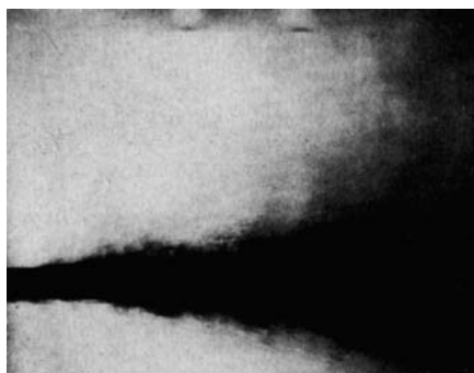
Fig. 5. Flashing jet 10X. Type B, D = 0.031 in., P = 120 lb./sq. in. T = 295^\circ\text{F} .
